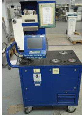
Object OP07: Calibration screwdriver BLM 0,1-1Nm / 0,5-6Nm / 6-36Nm Year 2003
