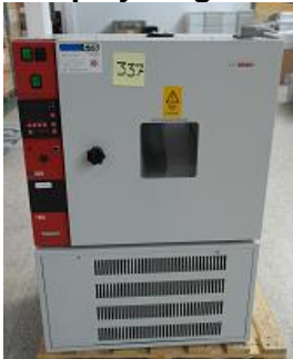
Object OP08: WTC Binder Type: 07053150402000 Temperature cycling -40° - +150°C
